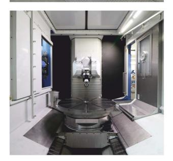
guarantees that the sizes of the final piece are maintained. This process involves the pre-grinding of the piece on the disc, measuring the size obtained with the probe, subsequent correction of the depth of cut if required and finally finishing. All steps are supervised by a software.
