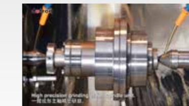
Grinding of consolidated spindle unit
