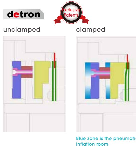
**detron** applies exclusive patented dual pistons to **multiply the pneumatic pressure zone** and **promote the clamping power**.
