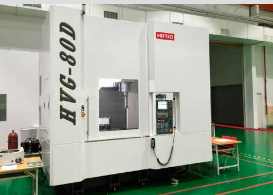
Vertical grinding machine in hydrostatic technology
