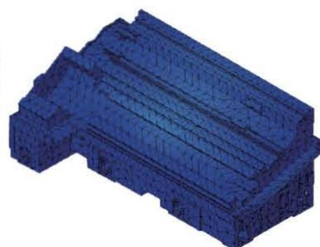
Physical rigidity are ensured for all AKIRA-SEIKI Turning Center in the primary design progress by advanced digital assay tool. All structural frames apply COSMOS system for analysis to optimize rigid mechanism foundation.
